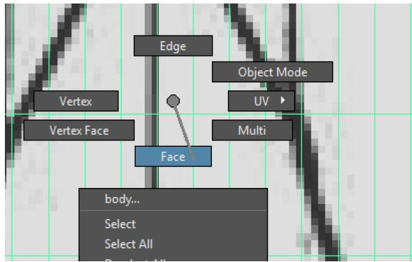
When deleting we want to delete through the model, to ensure this happens hold down shift whilst highlighting multiple faces.
