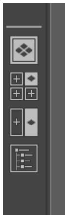
As you can see, the toolbar offers single view(Perspective), the 4-way view (perspective, front, side and top) a 2-way split (defaults to front and perspective) and the outliner panel hide/show option.
